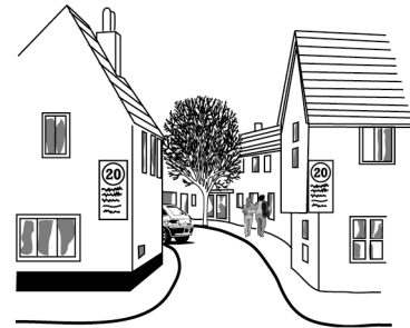
Gateway consisting of 'pinch point' of buildings
